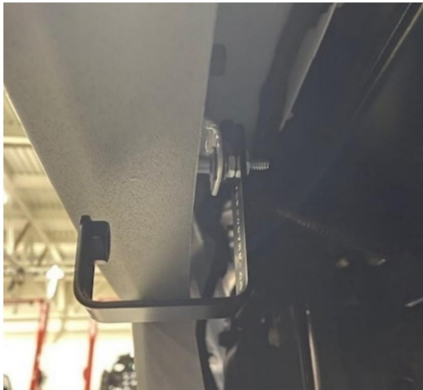
4. Place the foam pads provide on the backside of your license plate or directly onto the bumper cover to aid in preventing any squeaks and rattles between the front plate and the bumper.
